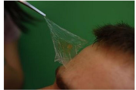
The patch of electronic skin consists of an array of electrical devices for monitoring the vital signs of the body
