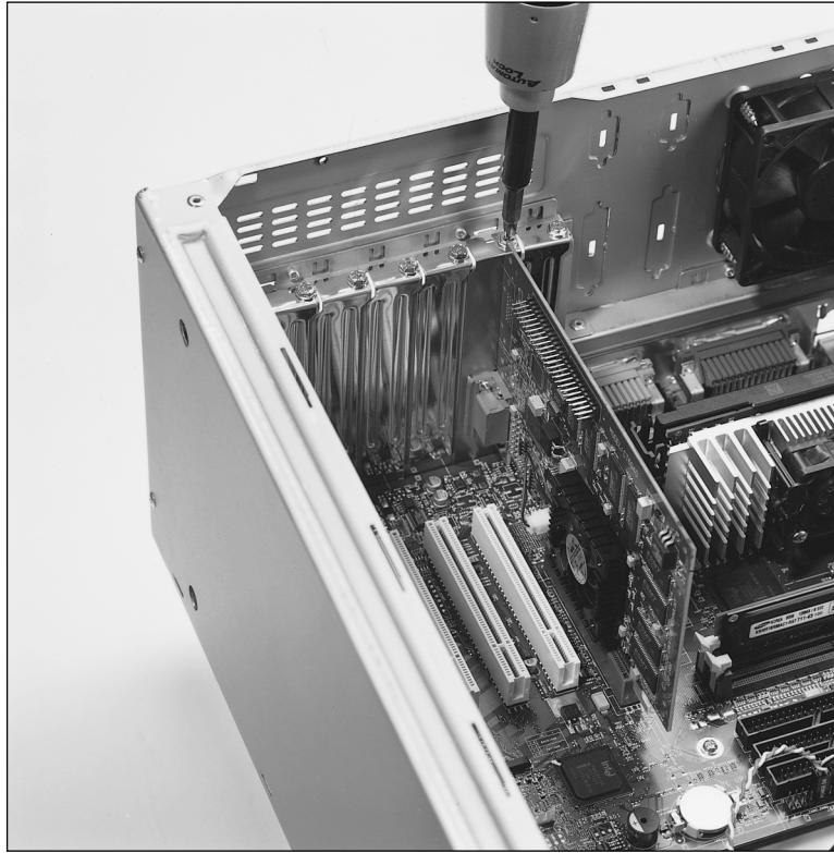
Figure 23.29 Installing the screw to retain the card. Motherboard courtesy of Intel Corporation.
