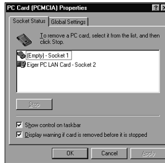
Figure 19.14 This notebook computer has a network card properly installed in its PCMCIA slots but not a modem. If the modem isn't pushed into the slot firmly, it will appear to be missing.
