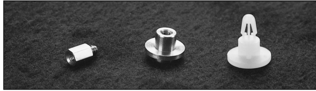
Figure 23.11 Various types of motherboard standoffs, used to support the board when installed in the chassis or motherboard tray.
