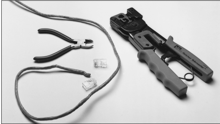
Figure 20.17 You'll need wire strippers, a crimping tool, UTP cable, and RJ-45 connectors to make your own 10BASE-T (100BASE-T) cables.
