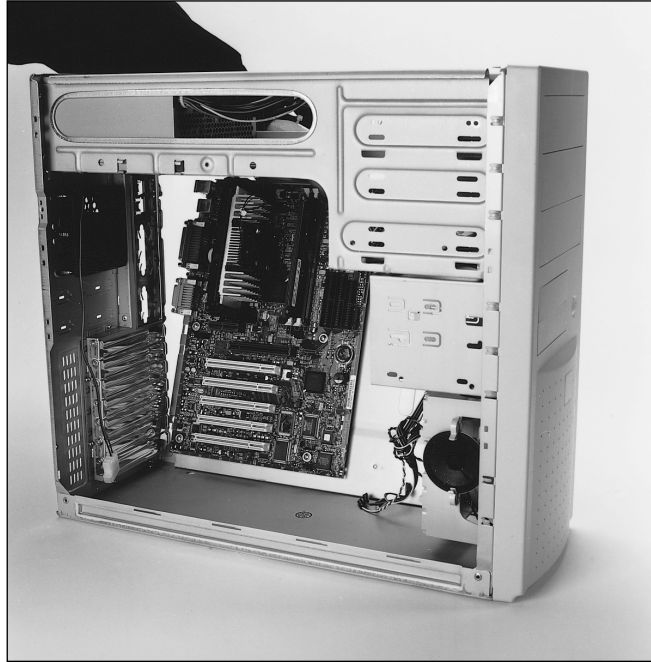
Figure 23.16 Installing the motherboard and tray into the chassis. Case courtesy of PC Power & Cooling, Inc. Motherboard courtesy of Intel Corporation.
