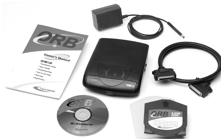
Figure 12.5 The external SCSI version of the Castlewood Orb drive comes with an HD-50 SCSI cable, an AC power pack, driver files on CD-ROM, one Orb disk with case, and a manual. As is typical with most SCSI drives, the SCSI host adapter is not included. Photo courtesy of Castlewood Systems, Inc.
