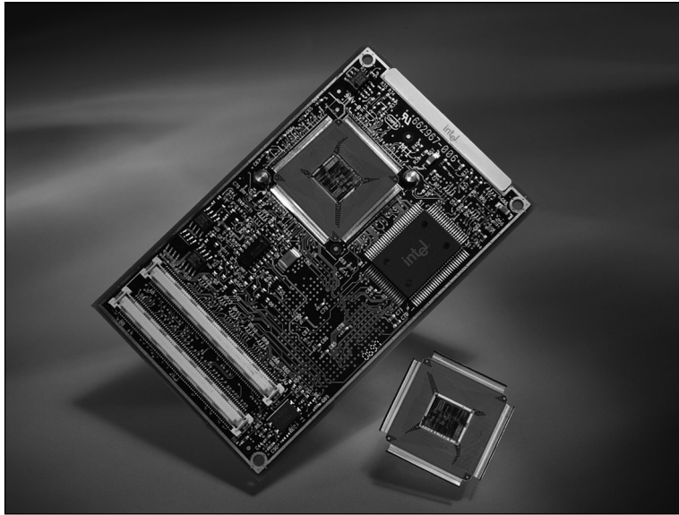
Figure 22.7 Mobile Pentium processors in mobile module or raw tape carrier package form. Photograph used by permission of Intel Corporation.
