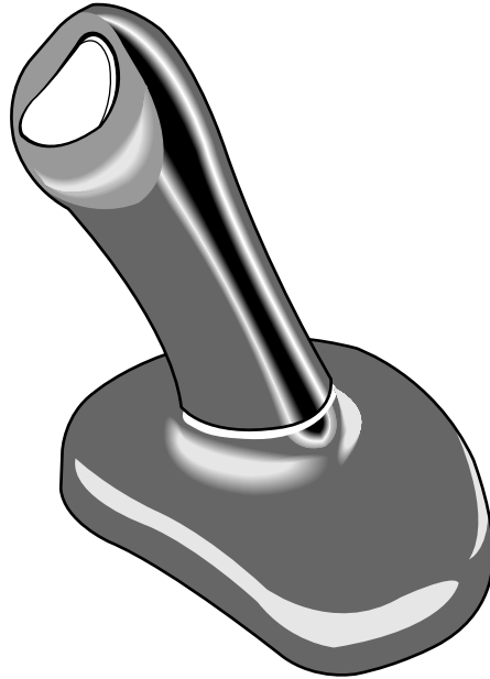
Figure 18.11 The 3M Renaissance Mouse combines an ergonomic shape with a standard mouse-movement mechanism.
