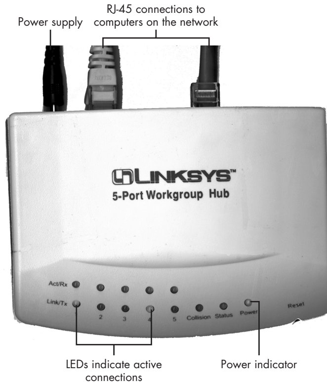
Figure 20.13 A typical 10BASE-T five-port workgroup hub. Connectors 1 and 4 are connected to computers (as shown by the lights at the front of the hub [bottom of the picture]). The light at right indicates the hub is receiving power from a AC/DC transformer “brick.”
