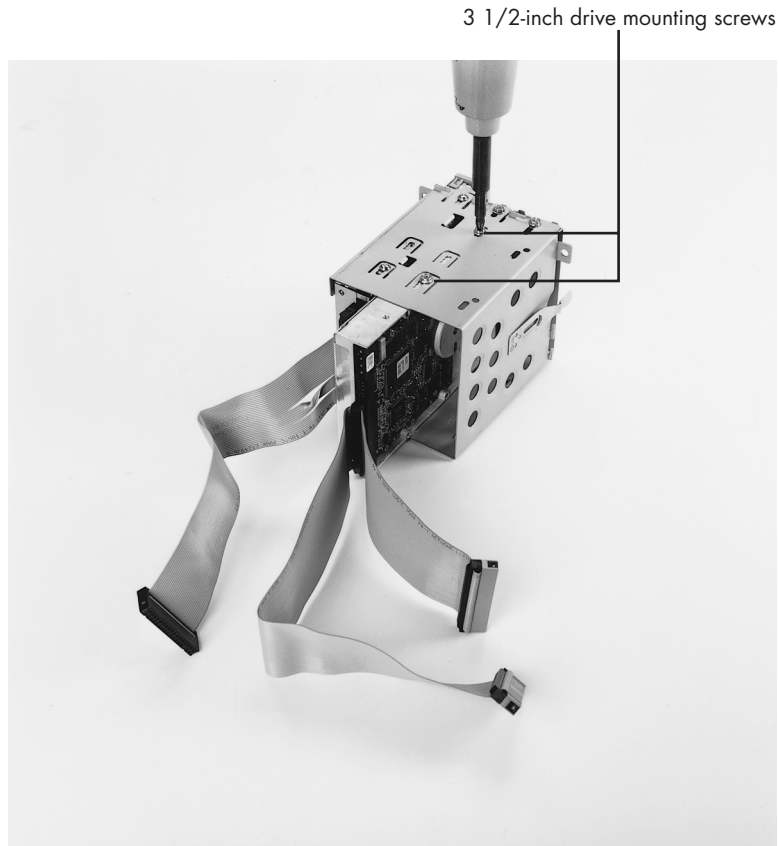
Figure 23.26 Use four screws to secure each drive to the drive cage. Chassis courtesy of PC Power & Cooling, Inc. Hard drive supplied by Micro X-Press.
